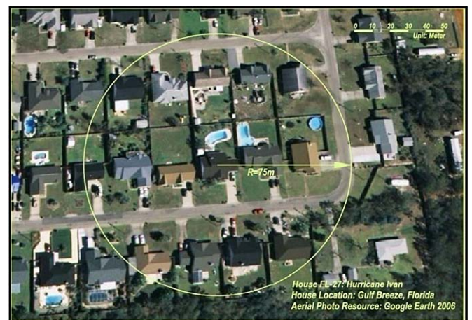
Fig. 3. Aerial view of the House FL-27 and neighboring houses (Courtesy of Google Earth). Circle indicates the extent of turntable for wind tunnel experiments.
