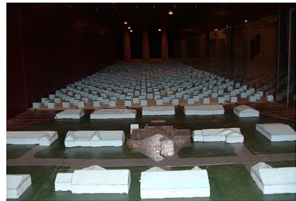
Fig. 8. The 1:50 scale model of House FL-27 and surrounding models installed on turntable.
