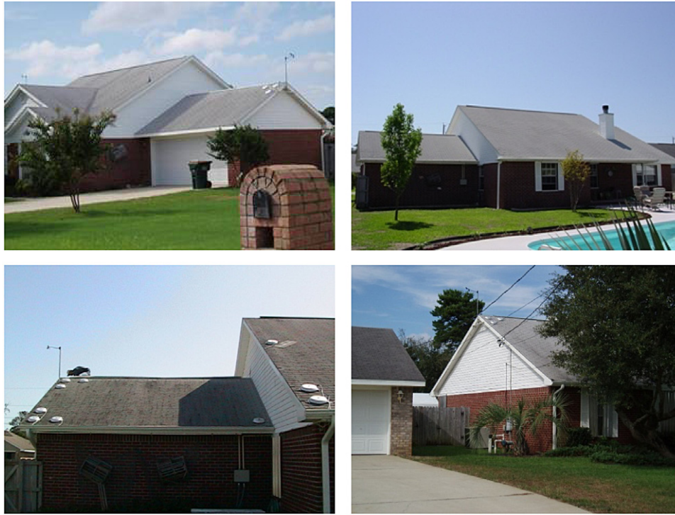
Fig. 4. Photographs of FL-27 showing anemometer location and pressure sensors.
